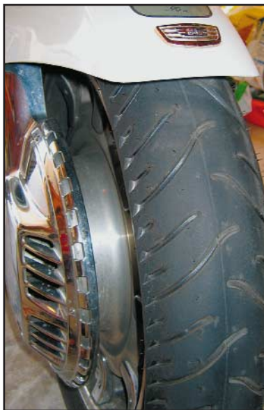
New tread pattern for the bias ply GL1500 tire, which is similar to the GL1800 radial tread.
